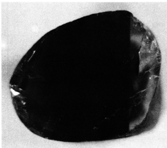
Fig. 2. Effect of \gamma -irradiation in topaz (second type): Crystal plate (001) cut perpendicular to the c -axis; sharp boundary between the brown and colourless part of the crystal.
